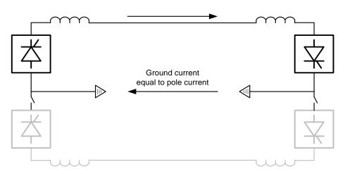
Figure 1.3 - Bipolar Configuration Operated as A monopole with Electrodes
