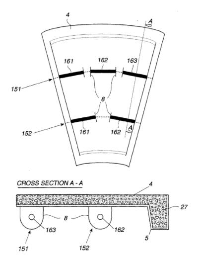
Figure 5.29 - Section Of An Electrode, Seen from Below, With A Ballast in the Form of Concrete Plate with Coated Side Walls and A Section along The Line A-A [60]
