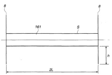
Figure 5.25 - Cylinder Shaped Sub-electrode Element Provided with Non-conducting Barriers [60]
