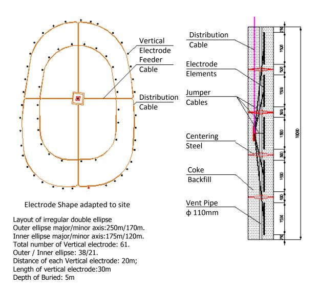
Figure 2.9 - Vertical Electrode of ±800kV HVDC Puer-Qiaoxiang Project with Rated Current 3125A
