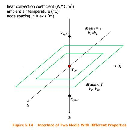
When the node is located at the interface between two media as shown in Figure 5.14, Equation 5.3-7 changes to [45]
