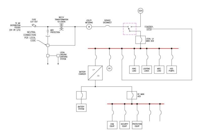
Figure 7.1 - Typical Single line Diagram
