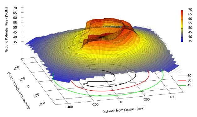
Figure 5.9 - Example of Calculated Ground Potential Rise near A Shallow Double Ring Electrode With A Portion of The Electrode Out of Service
