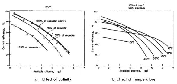
Figure 5.20 - Current Efficiency vs Available Chlorine Concentration using DSA Anodes [59]
