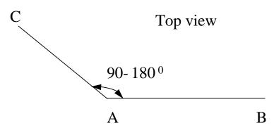
Figure 8.4 - Angle between current line and potential conductor
