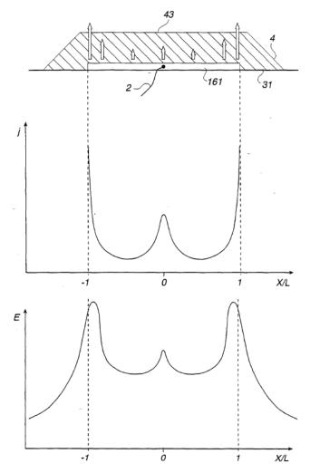
a) Side view of a sea electrode with a mesh type sub-electrode element and gravel layer ballast.
