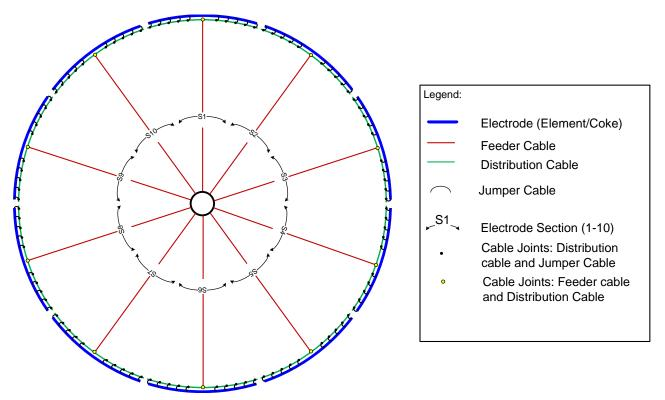
Figure 0.2 - Conceptual diagram showing a ring electrode connection
