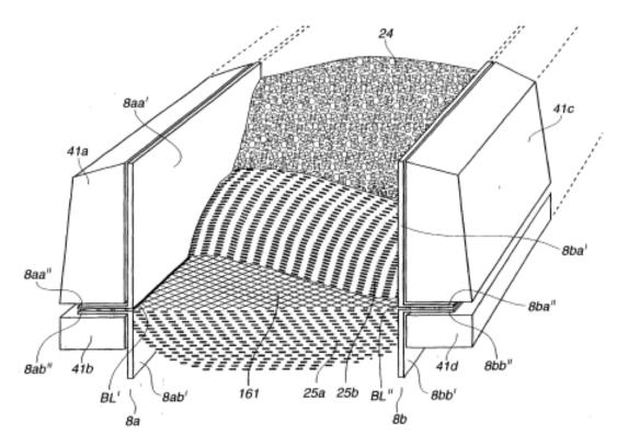
Figure 5.30 - A Sub-electrode Element Embedded in a Backfill [60]
