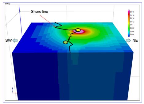
Figure 3.11 - Calculated potential RISE due to current injection at Forsmark (Figure 3.10) into the resistivity model [12]
