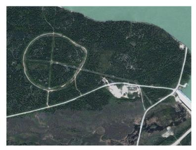
Figure 2.4 - Land Electrode (Manitoba Bipole 1 – Radisson)
