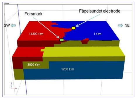
Figure 3.10 - Regional resistivity model around the Fågelsundet electrode based on open-file data [12]
