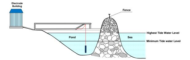
Figure 2.16 - Conceptual Plan and Profile Views of a Pond Electrode
