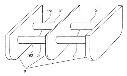
Figure 5.26 - A Pair of Cylinder-shaped Sub-electrode Elements with Non-conducting Barriers, also Serving as Mechanical Supports [60]
