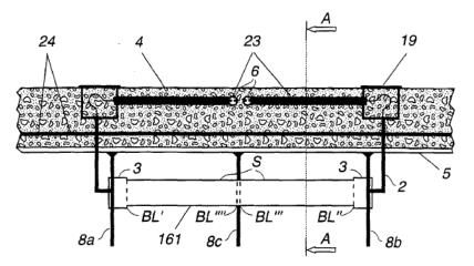
(a) Side view of a part of an electrode with sub-electrode elements according to Figure 5.26 arranged at an armored concrete plate
