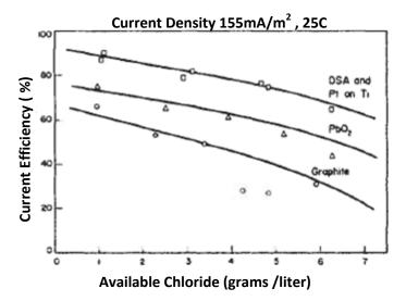
Figure 5.19 - Current Efficiency vs. Available Chorine Concentration in Seawater for Different Electrode MaterialS [59]
