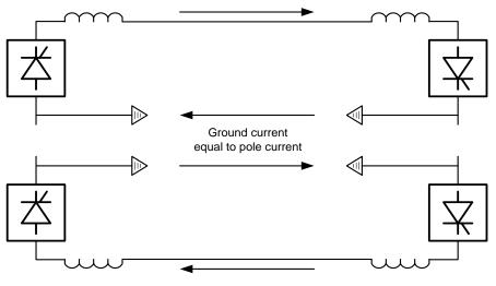
Figure 1.1 - Monopole Configurations with Electrodes
