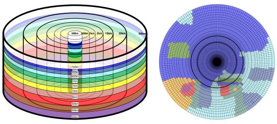
(a) A circular cylindrical volume resistivity model (7 circles x 11 layers) (b) Resistivity assigned for soil near the electrode for the layer where the electrode is buried
