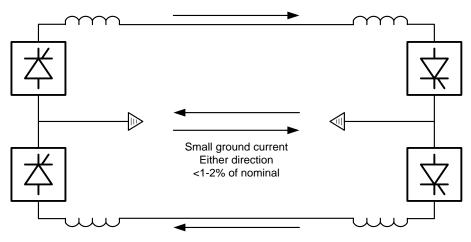
Figure 1.2 - Bipolar Configuration with Electrodes
