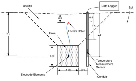
Figure 8.1 - Soil Temperature Measurement Diagram
