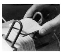
Useful when beaming long warps. They are placed in each section every 5 or 10 yards (meters) to prevent uneven build-up of threads and keep uniform tension in the warp. They all have to be placed in the same turn
