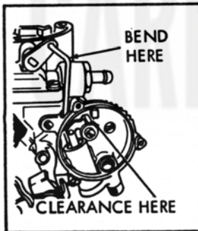
CHOKE PISTON LINKAGE ADJ. Fig.4
