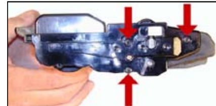
A. Remove the 3 screws on the right end cap.
