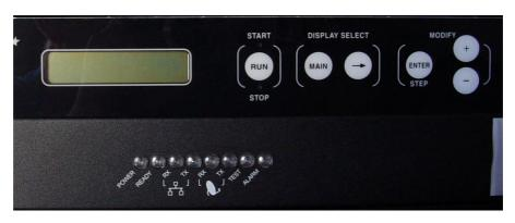
warning lights stop flashing on the main control panel and the dash board, you will know that the antenna is in the "stowed" position.
