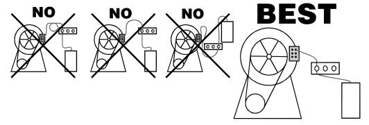
**Note 1:** As shown in Figure 2, all tanks, pumps, and tubing must be lower than the injection point on the machine and must not dribble chemicals into the machine, nor leak chemicals externally onto any portion of the machine or its surroundings.
