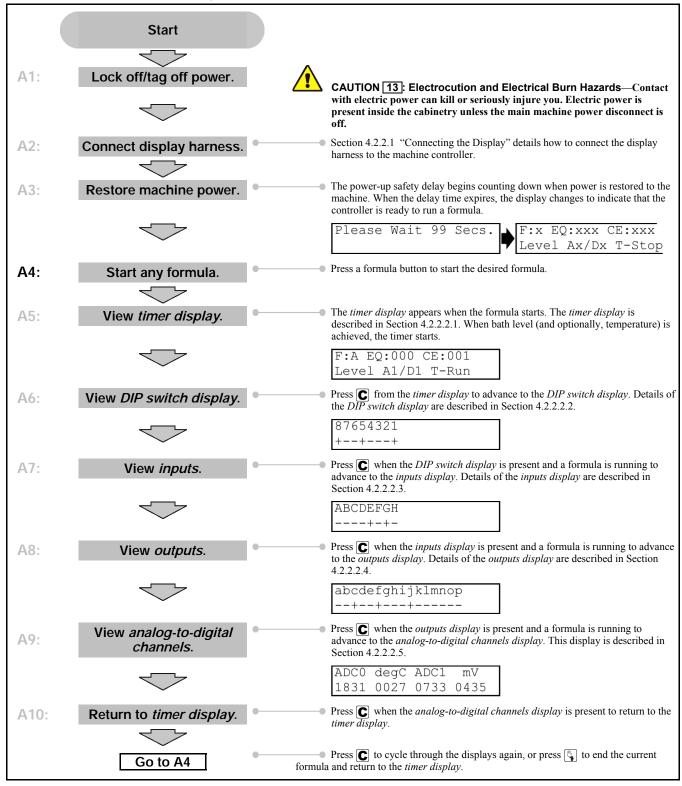
4.2.2.2.1. **Timer Display**—When power is supplied to the machine, the display shows the time remaining in the power-up safety delay and the *In Progress* light flashes. When you start a formula, the
