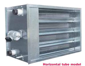
There are two distinct Aeromix® coil types available, most easily differentiated by the tube orientation. The vertical tube Aeromix® coil is a copper spiral fin design used in larger face area applications, up to 88 square feet. The smaller horizontal tube coil is an aluminum plate fin design used in applications up to 24 square feet in face area.
