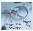
fire the cartridge. Tighten the set screw and replace the grip and grip screw.
