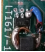
Figure 15: Custom wire fix with cut on-board wire
