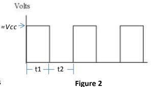
capacitor discharge time through only Rb. In comparing the above equations for t1 and t2 it can be seen that since both Ra and Rb are positive real values it is impossible for t1 to be less than t2. Thus only duty cycles of >50% can be obtained.
