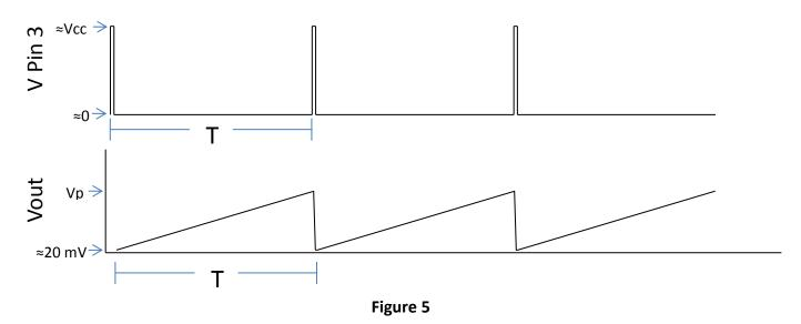
the collector and emitter of Q1. Once the output of the LM555 at pin 3 returns to a low state Q1 again goes into cutoff and the charging process of C1 starts again until the output of the LM555 returns high.
