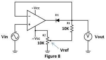
Vref can be a positive or negative voltage depending on the waveform design needs. In Figure 8 Vref is a positive value because R2 is attached between +Vcc and ground. R2 could also be attacked between-Vcc and ground, in which case a negative Vref can be achieved.
