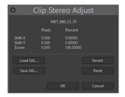
The buttons underneath the controls allow you to Import or Export the Stereo Adjust data to use the values in other applications, such as Fusion and Dimension.
