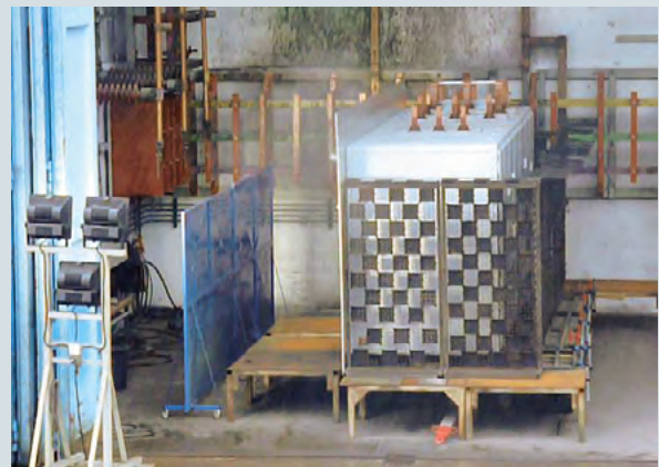
Fig. 54 Internal arc test at an independent laboratory
