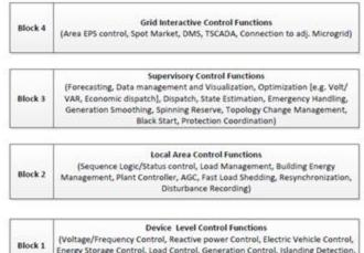
Iock 1 (Voltage/Frequency Control, Reactive power Control, Electric Vehicle Control, Energy Storage Control, Load Control, Generation Control, Islanding Detection, Fault Protection)
