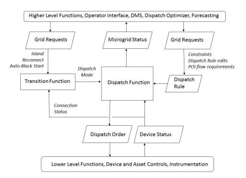
Figure 5. MMC core functions
