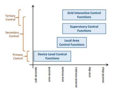
Figure 3 Control Elements Time of Action
