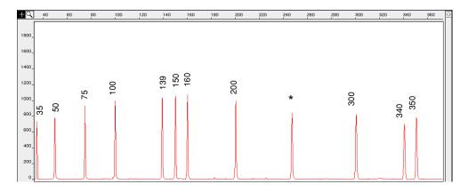
**Figure 5-1** Electropherogram of the GeneScan-350 size standard run under denaturing conditions on the ABI PRISM 310 Genetic Analyzer. Fragments were run using the POP-4 polymer at 60 °C.
