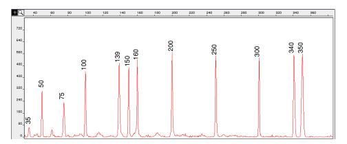
**Figure 5-2** Electropherogram of the GeneScan-350 size standard run under non-denaturing conditions on the ABI PRISM 310 Genetic Analyzer. Fragments were run using 3% GeneScan Polymer at 30 °C.
