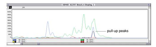
Figure 3-6 Characteristic appearance of bleedthrough peaks
