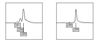
**Figure 6-2** Comparison of the amounts of stutter in dinucleotide (left) and tetranucleotide (right) repeat loci. Each locus is homozygous, with the largest peak in each picture representing the "true" allele.
