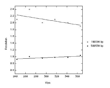
**Figure 2-10** Resolution vs. electrophoresis voltage for different-sized GeneScan-2500 fragments, 2.5% GeneScan Polymer in 41-cm capillary at 30 °C
