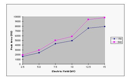
Figure 2-7 Peak area vs. injection voltage for two different-sized fragments (150 bp and 340 bp
