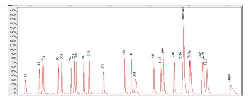
**Figure 5-10** Electropherogram of the GeneScan-2500 size standard run under non-denaturing conditions on the ABI PRISM 310 Genetic Analyzer. Fragments were run using 3% GeneScan Polymer (GSP) at 30 °C.
