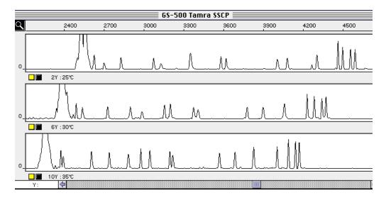
**Figure 7-1** GeneScan-500 [TAMRA] run in 3% GeneScan Polymer with 10% glycerol with 1X TBE buffer,  $L_t = 47$  cm, 13 kV electrophoresis voltage
