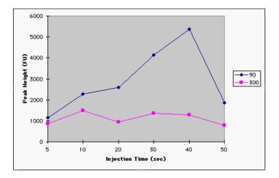
Figure 2-3 Peak height vs. injection time for two different-sized fragments (90 bp and 300 bp)
