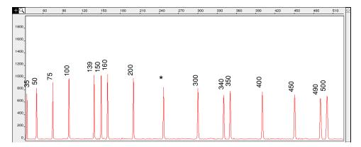
**Figure 5-5** Electropherogram of the GeneScan-500 size standard run under denaturing conditions on the ABI PRISM 310 Genetic Analyzer. Fragments were run using the POP-4 polymer at 60 °C.
