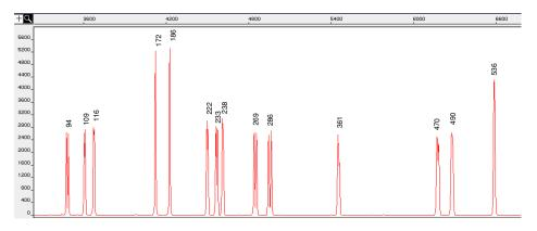
**Figure 5-9** Electropherogram of the GeneScan-2500 size standard run under denaturing conditions on the ABI PRISM 310 Genetic Analyzer. Fragments were run using the POP-4 polymer at 60 °C.
