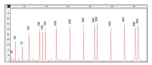
**Figure 5-6** Electropherogram of the GeneScan-500 run under non-denaturing conditions on the ABI PRISM 310 Genetic Analyzer. Fragments were run using 3% GeneScan Polymer (GSP) at 30 °C.
