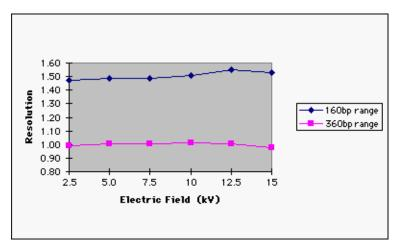
Figure 2-8 Resolution vs. injection voltage for different-sized fragments
