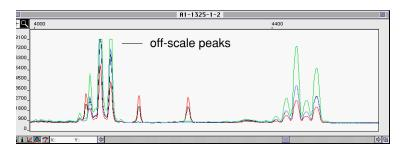
Figure 3-4 Raw data from an overloaded sample
