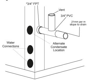
\* Some units include a painted drain connection. Using a threaded pipe or similar device to clear any excess paint accumulated inside this fitting may ease final drain line installation.
