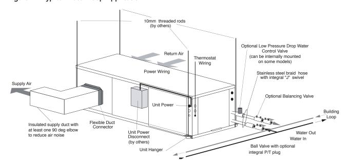
Figure 12: Typical Water-Loop Application
