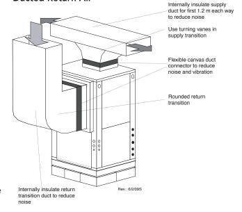
**Sound Attenuation for Vertical Units** - Sound attenuation is achieved by enclosing the unit within a small mechanical room or a closet. Additional measures for sound control include the following:
