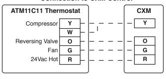
Field Wiring -----Factory Wiring -----
