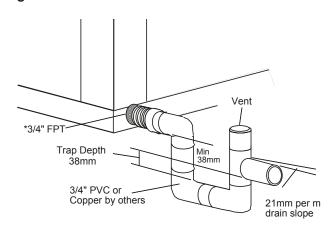
\* Some units include a painted drain connection. Using a threaded pipe or similar device to clear any excess paint accumulated inside this fitting may ease final drain line installation.
