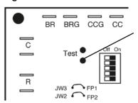
Short test pins together to enter Test Mode and speed-up timing and delays for 20 minutes.
