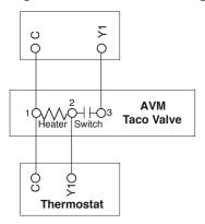
Figure 23: Taco SBV Valve Wiring
