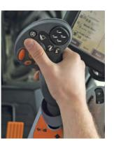
• Rear linkage raise/lower. To activate front linkage raise/lower, push the button on the rear of the CommandGrip controller simultaneously with the raise/lower function.
