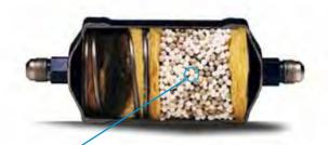
Some imitation driers may use granular or 'bead' technology where desiccant beads rub together as refrigerant passes through, causing the risk that fine pieces of the beads could be passed into the system.
