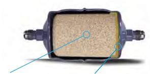
Thermo King driers use a full wrap final filter pad that imitation driers do not match. The full wrap feature provides an optimum end cap seal so that no appreciable physical particulate material can escape the drier.
