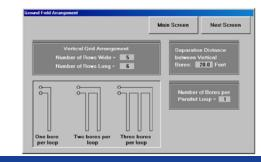
"Adequate separation is required to prevent short and long term heat storage effects in loop fields. This is especially true when with clay and impermeable rocks are present. Water movement will be minimal and heat will be significant in typical commercial /institutional buildings if the bores are located less than 20 feet apart."
