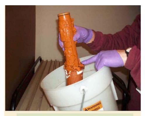
Iron sludge from a blocked strainer
