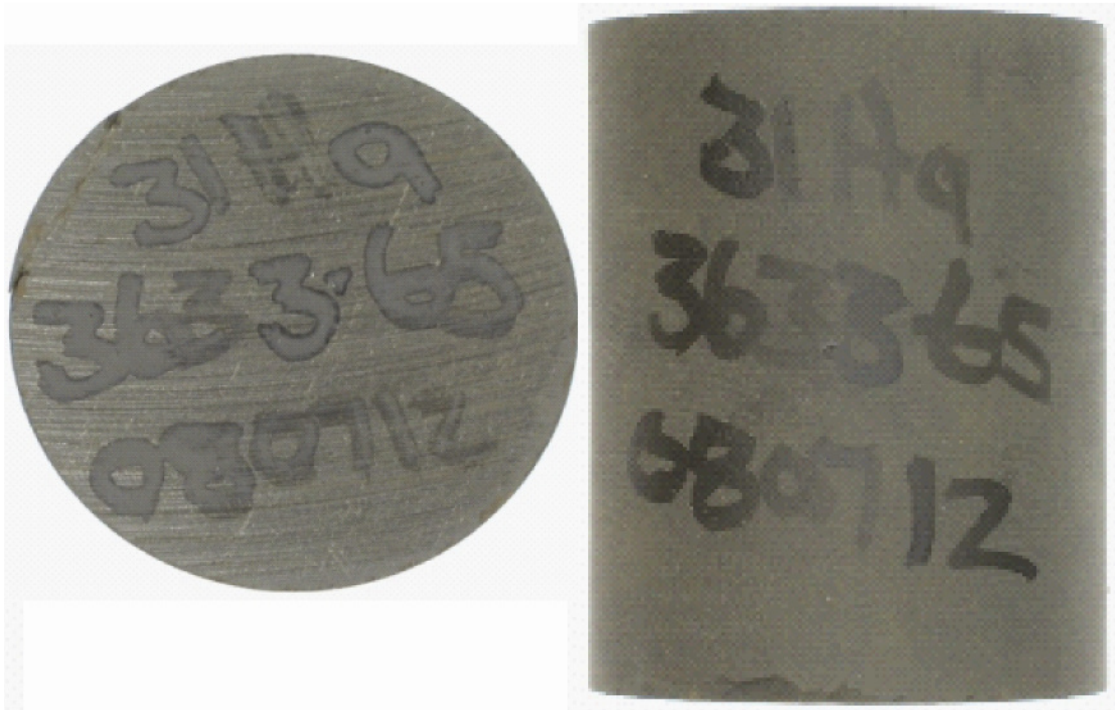
Figure 2.16: Sample 31Ha, a typical dark, organic-rich Barnett shale sample.
