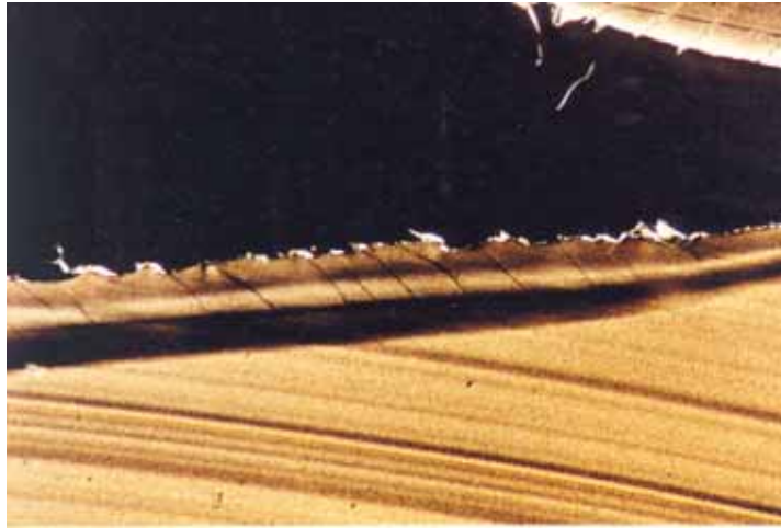
Figure 1. Craze in peel-separated weld. Microsection viewed with crossed polarizing filters.
