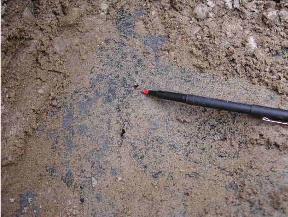
Figure 8. 5 mm punctures in landfill cap made by large rounded rock.
