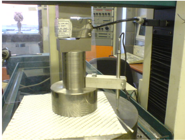
Figure 5.1: Fabric compression rig
