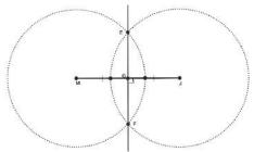
Use the diagram to guide you in constructing the perpendicular of the following line segments. Mark the right angle with the correct symbol for right angles. Indicate the segments are congruent by using slash marks.
