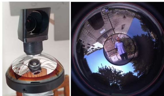
Figure 3 PAN-ROVER head and image example
