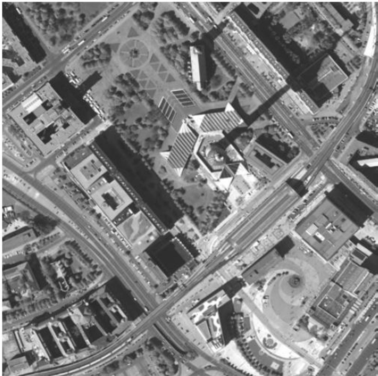
Figure 2.33 Rectified ADS 40 image.
