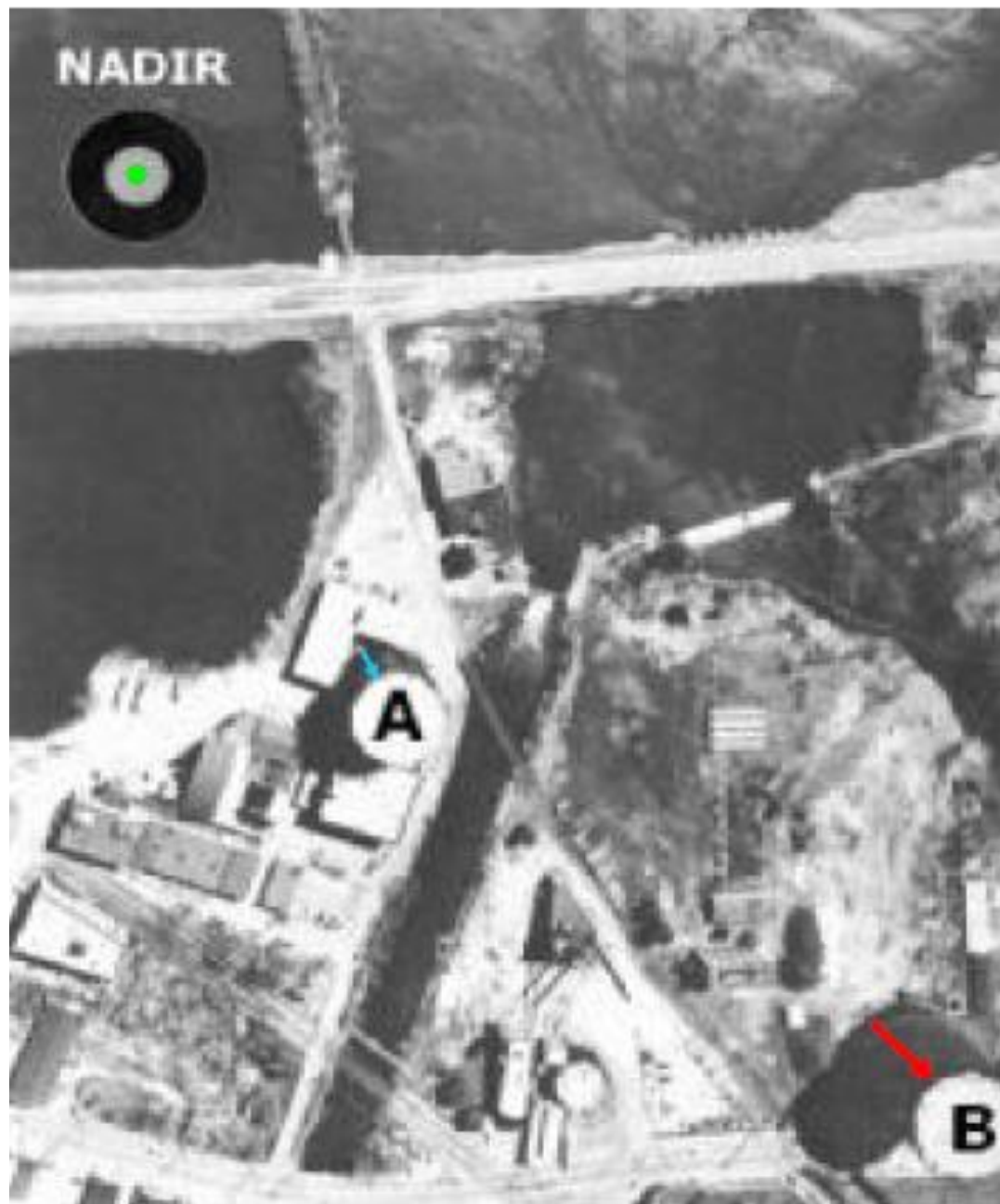
Relief displacement from Nadir (enlarged)
