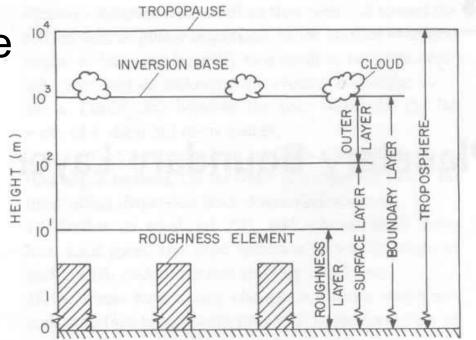
Figure 4.1 Schematic of the planetary boundary layer (PBL) as the lower part of the atmosphere.
