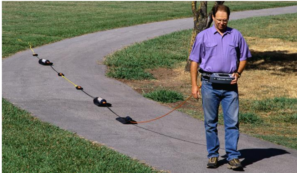
Figure 2-4: The OhmMapper capacitive-coupled electrical resistivity system. From www.geometrics.com
