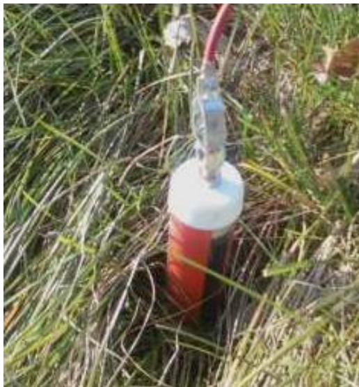
Figure 2-6: Non-polarizing Cu-CuSO 4 porous pot electrode used in SP surveys
