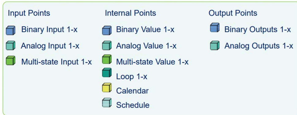
Figure 9. An example of a BACnet device [32]
