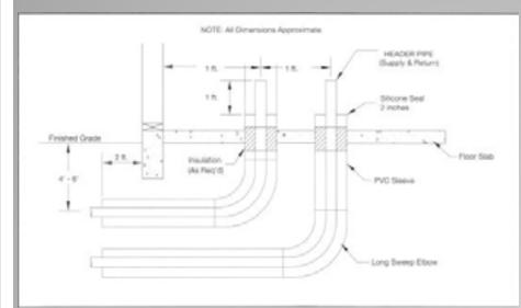
Long Sweep Elbows for Pipe Bends!... Proper pipe sleeve sizing and configuration will make it a lot easier to place geothermal HDPE supply/return header pipes later.
