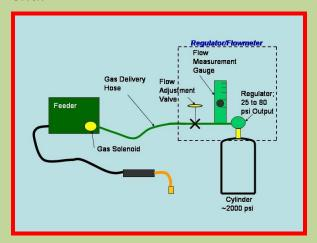
To keep flow at the preset level the gas pressure in the cylinder regulator will be between 25 and 80 psi. Flowgauge regulators (those with a flow calibrated pressure gauge) operate in this pressure range as well.) However to flow
