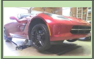
The car does not have to be jacked up very high as the skid pads are close to the front. It is advised to put jack stands under the car whenever it is jacked up. In this case they can be placed under the front cradle as defined in the Owner's Manual. Since you will not be going under the car very far just placing the jack stands under the outer ends of the cradle it all that is necessary.
