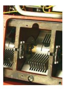
**EK Receiver,** top view, showing tube sockets, IF transformers and chassis compartments. Image courtesy Bo Samuelsson
