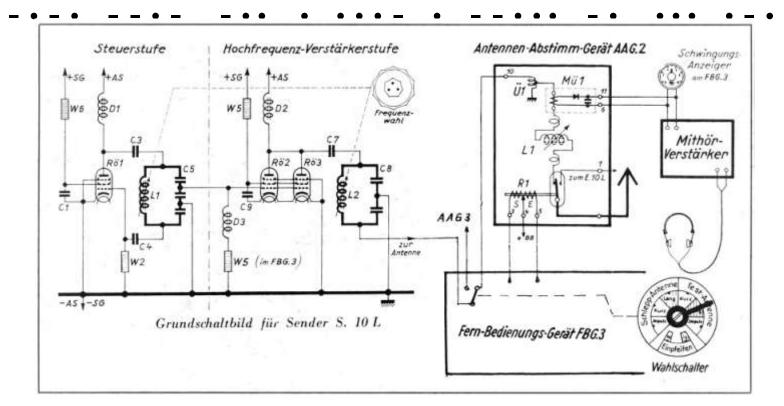
Note 1: Connections from TX and RX via Ant. Control Unit (FBG.3) to ATU (AAG.2) are  $60\Omega$  coax.
