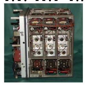
**EK** front panel frame & tuning dial mechanism with 4 preset cams. Image courtesy LA6NCA
