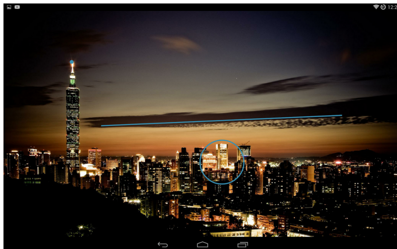
Figure 3.6 Picture lock. The unlock gesture consists of moving the finger across the distinctive skyline and touching the building in the middle, as marked by the blue lines. Courtesy of Google Play
