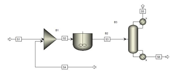
4.40. Click on the **Heat Exchangers** sheet of the **Model Palette**. Click the **Heater** button. Addit to the flowsheet below the reactor.
