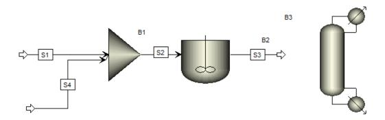
4.33. Reconnect the destination of stream **S3**. Either right-click **S3** and select **Reconnect Destination** or double click the white arrow at the right end of **S3**, and then click the red arrow pointing into the column.
