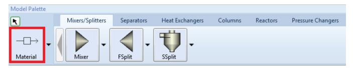
4.16. Click on the flowsheet area in two different spots (one for stream source and again for stream destination). A stream **S1** is drawn in the flowsheet area. The mouse is still in the insert mode. Clicking in the flowsheet area again will make another stream.
