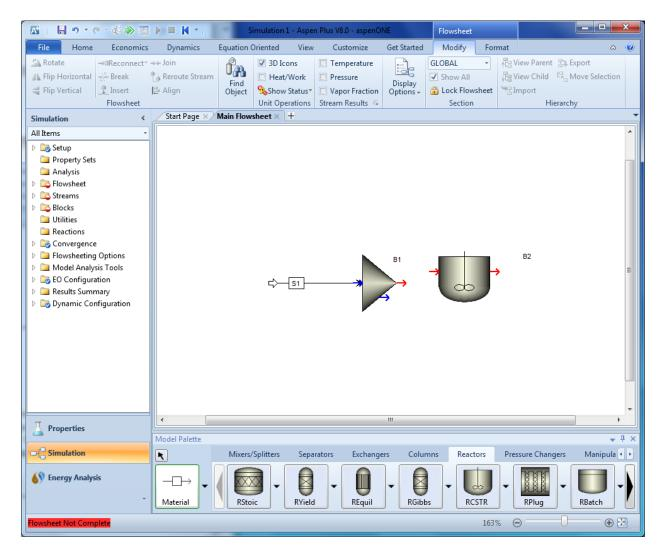
4.28. Click on the red arrow pointing out of **B1** and then click the red arrow pointing into the reactor. Now, **B1** and **B2** are connected with a stream. Add an effluent stream by clicking on the red arrow coming from the reactor and then click on a blank spot on the right of **B2**. The flowsheet should look like the screenshot below. The label for **S3** is hidden because the **B1** and **B2** are so close together.
