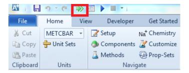
4.12. When the **Next Input** button is clicked after the property methods have been specified, this sheet appears. No further action is required from the user for the binary interaction parameters because they have been filled up automatically.
