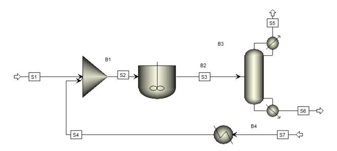
4.43. Join the streams to complete the recycle loop. Click on stream **S6**, press and hold the **Ctrl key** on your keyboard, and then, click **S7**. Then, release the **Ctrl key** on your keyboard. Both **S6** and **S7** are selected. Right-click one of them and select **Join Streams**.
