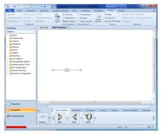
4.17. Cancel insert mode. To exit the insert mode, click the **Cancel insert mode** button (outlined in the red box below) in the **Model Palette**. Alternatively, right-click on the main flowsheet to cancel insert mode. Note that the cursor changes shape when you enter or exit insert mode. It is a "plus" sign in insert mode, and an arrow when not in insert mode.
