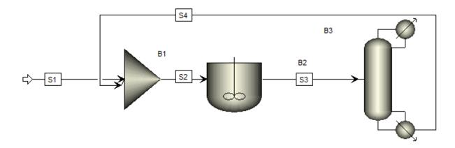
4.36. Move the recycle stream by clicking and dragging so that the stream is below the blocks. Having a clean flowsheet becomes very important when there are many blocks and streams.
