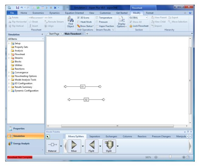
4.19. Delete **S2** by right-clicking it and selecting **Delete Stream**. Streams can also be deleted by clicking on the stream and pressing the **Delete Key**.
