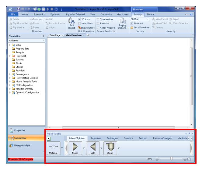
4.15. Create a stream in the flowsheet. Click on the **Material** button (outlined in red below) in the **Model Palette**. Now, the mouse is in the insert mode.
