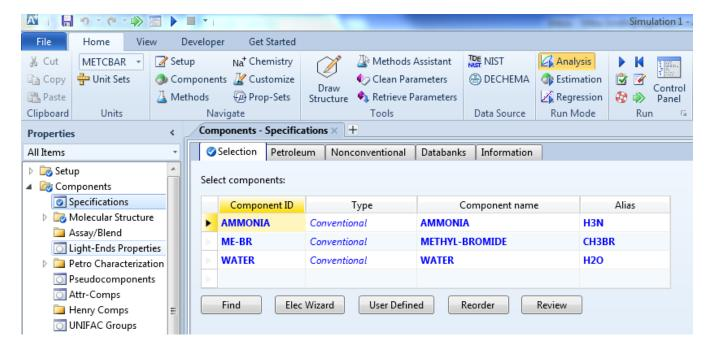
4.09. Specify the property methods to be used in the simulation by clicking on the **Methods** button in the **Navigate** group in the **Home** tab of the ribbon. Alternatively, click the **Methods** node in the navigation pane.
