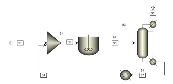
4.45. Rename a block. Right-click on **B2** and select **Rename Block**. Enter a new name, like **REACTOR**. Both streams and blocks can be renamed in this way. Alternatively, a block can be renamed by clicking on the block and pressing **Ctrl+M**. A stream can be renamed in a similar way.
