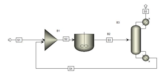
4.38. Add a heater for the recycle stream **S4**. Break the recycle stream **S4** by right-clicking on it and selecting **Break Stream**.
