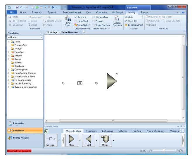
4.22. Connect the stream to the block. Right-click on the stream and click **Reconnect Destination**.
