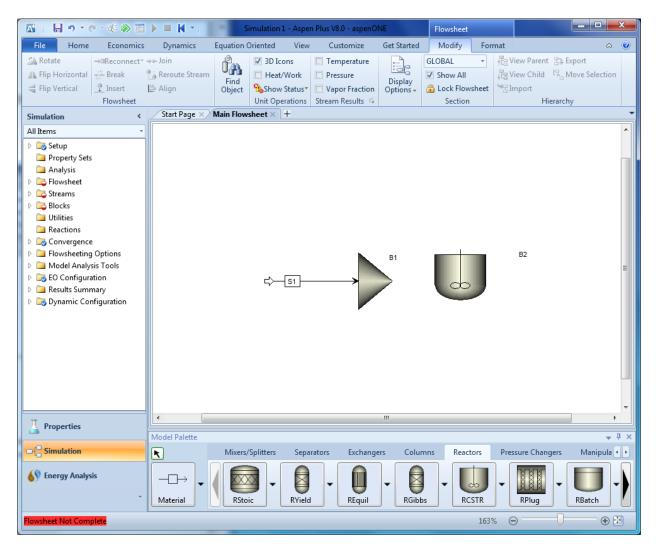
4.27. Connect the mixer to the reactor. Click on the **Material** button in the **Model Palette**. Doing so will show all available inlet and outlet ports. Again, red ports are ports that require stream connections, blue are optional.
