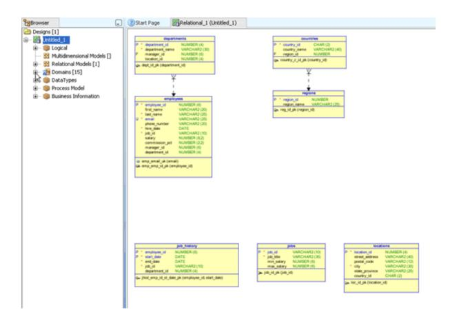
10. Note that domains are used in data type definitions - domains like VARCHAR\_0\_0\_20 or NUMERIC\_4\_0\_0 are created c data types (used in column definitions) are aggregated into domains. These names can be changed. Double-click NUME
