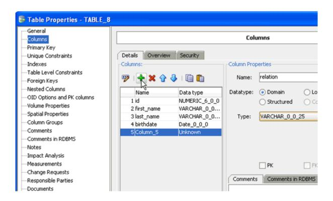
9. Enter gender for the Name. There is no character domain with the length of 1 so you can use logical type. SelectLogical select VARCHAR from the Type drop list, enter 1 for Size and select CHAR for Units. Then click the Create Column
