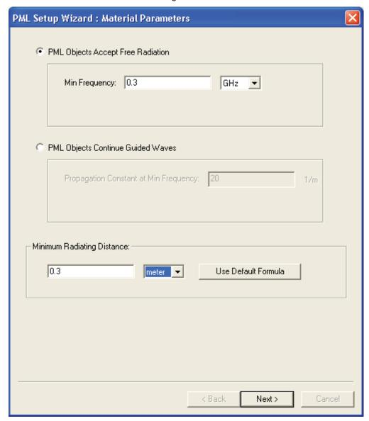
**8** Set the Minimum Frequency to 0.3 Ghz, and the Minimum Radiating Distance to 0.3 meter, as shown.
