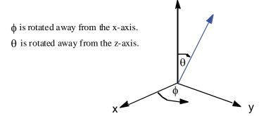
When HFSS evaluates the radiated fields, it needs at least two directions along which to plot the fields. Therefore, if the step size for phi is zero, then the step size for theta must be greater than zero, and vice versa. This ensures that the fields are plotted in at least two directions.
