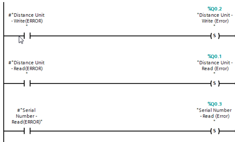
Figure 21: Main[OB1] program block – Network: Error handling of used acyclic read / write services.
