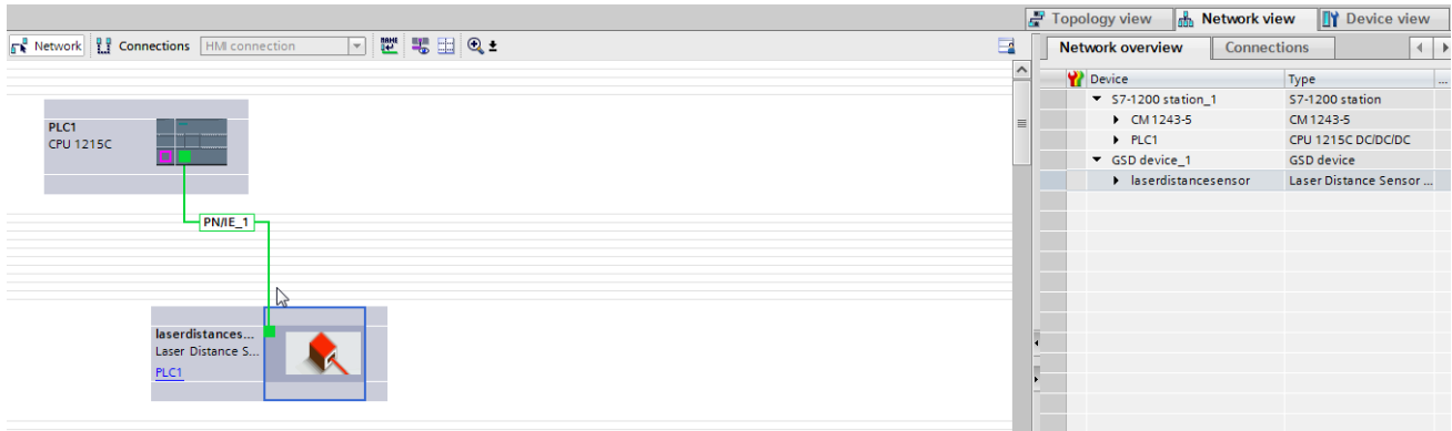
Figure 4: Network view – Overview of projected PLC and IO devices (without definition of the device port). Network devices: Siemens PLC CPU 1215 and Dimetix Laser Distance Sensor.
