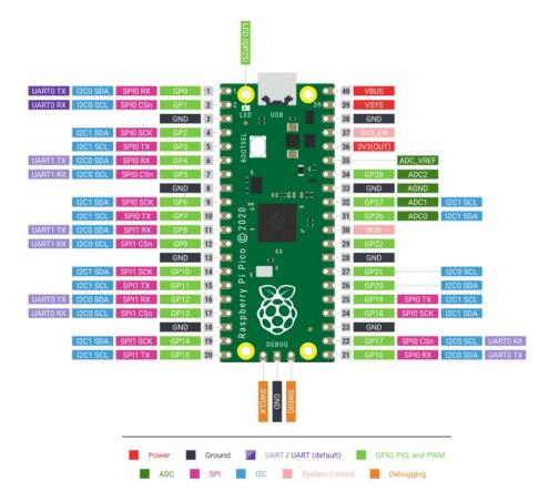
There are two I2C peripherals available, I2C0 and I2C1, two SPI peripherals, SPI0 and SPI1, and two UART peripherals, UART0 and UART1. You can assign any of these to the pins on which they are available. So for example, you can use GP0/GP1 for I2C0, and simultaneously use GP2/GP3 for I2C1, but you cannot use GP0/GP1 together with GP4/GP5 for I2C use, because they are both usable only with I2C0.
