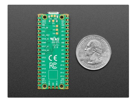
On the slim green board is minimal circuitry to get you going: A 5V to 3.3V power supply converter, single green LED on GP25, boot select button, RP2040 chip with dual-core Cortex M0+, 2 MegaBytes of QSPI flash storage, and crystal.
