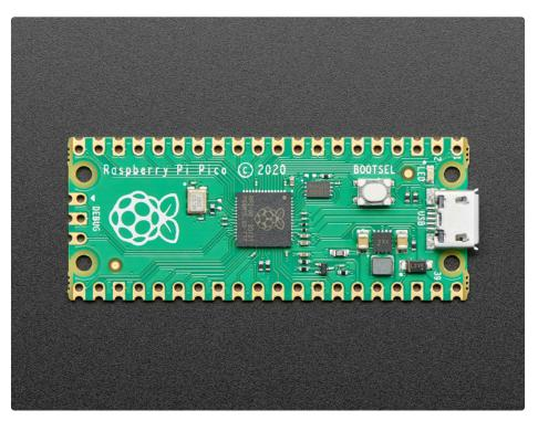
The Raspberry Pi foundation changed single-board computing when they released the Raspberry Pi computer (https://adafru.it/Qa1), now they're ready to do the same for microcontrollers with the release of the brand new **Raspberry Pi Pico**. This low-cost microcontroller board features a powerful new chip, the **RP2040**, and all the fixin's to get started with embedded electronics projects at a stress-free price.
