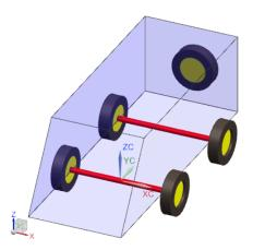
When the front left wheel gets inserted into the car assembly, this point P gets placed at (950, 0, 0). So, if comp is the FRONT\_LEFT\_WHEEL component, then comp.Position is (950, 0, 0). Similarly, the REAR\_LEFT\_WHEEL component has Position = (950, 2000, 0).
