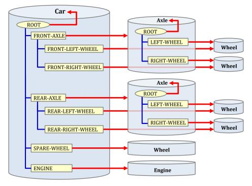
So, for example, as you can see, the axle part is the prototype corresponding to each of the components FRONT\_AXLE and REAR\_AXLE. Or, looking at it the other way around, FRONT\_AXLE and REAR\_AXLE are occurrences of the axle part.
