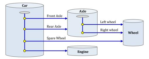
This diagram accurately reflects the structure of the data stored in NX. Notice that the wheel part is stored only once, even though the car has five wheels (the four main ones and a spare).
