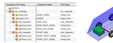
As you can see, the car consists of an engine (the green block), an exterior shape (the blue thing), two axles, and a spare wheel. Each axle consists of a shaft and two wheels. The exterior shape is a sheet body in Car\_Assembly.prt, so you don't see it in the Assembly Navigator. Similarly, the red shaft is a solid body in Axle\_Assembly.prt, so you don't see this, either.
