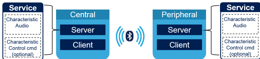
Figure 6. BlueVoice Profile GATT role assignment in a bidirectional system
