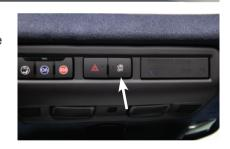
► To turn the systems on or off, press the **R** Sensors Disable button on the overhead console with the vehicle off.
