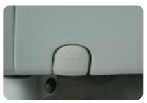
To open the hood, pull the hood release handle (shown above) located on the lower-left side of the instrument panel.
