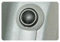
Your vehicle may be equipped with an outside power mirror control that adjusts the passenger-side mirror. The control is located on the driver door panel, above the power window buttons. Adjust the passenger-side mirror by pressing the edges of the control pad to move the mirror in the direction that you want it to go. The ignition must be ON.
