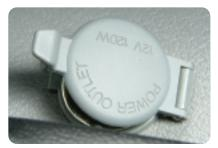
To use it, remove the protective cap and plug in the accessory. Replace the cap when not in use. (See your Owner Manual for important safety details.)
