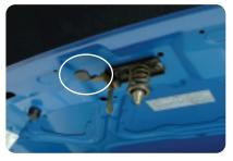
Lift the hood and release the hood prop from its retainer on the underside of the hood. Place the hood prop into the slot on the inner fender.
