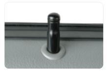
To prevent accidental lockouts, this function will not operate when the driver door is open, and the driver door itself will not lock when it is open.
