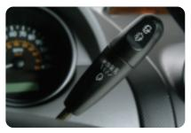
The lever on the right side of the steering column operates the front and rear windshield wipers. Move the lever to the following positions to operate the front wipers:
