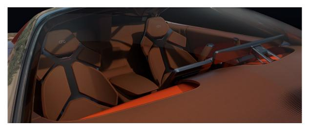
As for the interior, the two-seats-only formula offers two sporty but surprisingly comfortable seats with a special design featuring cushions fitted to a carbon structure so that driver and passenger are almost "lifted up" by the seat frame, thus ensuring comfort without sacrificing wraparound and restraining functions.
