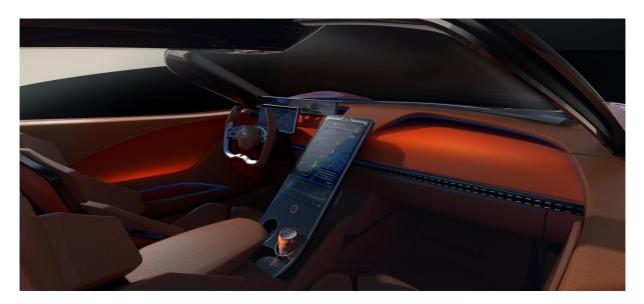
The dashboard is designed in two parts divided by an aluminum slat, which channels the air flows from the air conditioning: the upper part is a large leather wing, visually reminiscent of a horse saddle that joins up with the panels, while the lower part is made of Kult fabric in a dashing colour, in this case orange, to convey freshness, sportiness and also material innovation.
