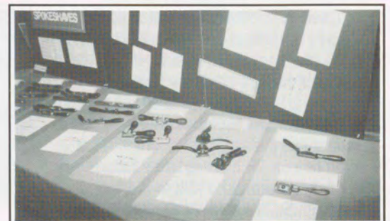
Judges Choice: Specialty spoke shaves with removable or repositionable handles, by Tom Lamond.
