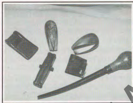
French tools for splitting, sizing width and thickness.
