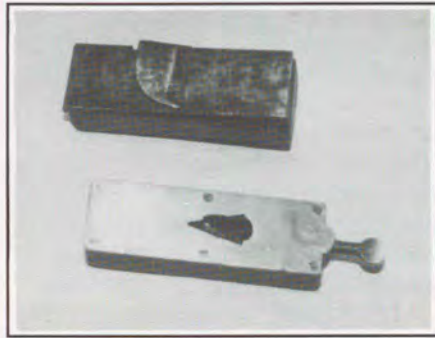
English tools for sizing width and thickness.
