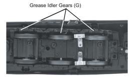
Figure 7. Greasing The Idler Gears
