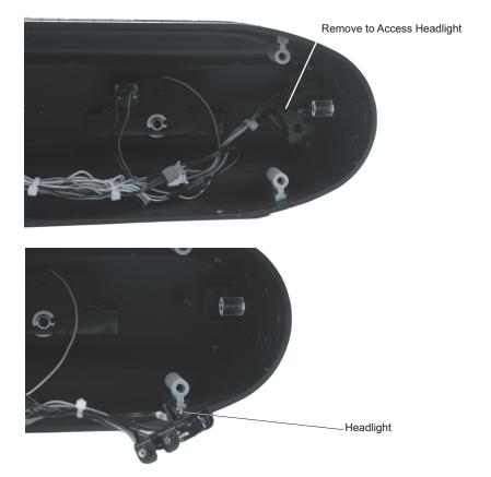
Figure 8. Removing the Headlight
