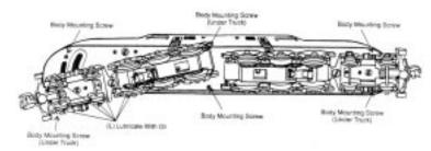
Figure 7: Lubricating The Truck
