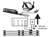
Figure 5: Wiring Up A Bell Button
