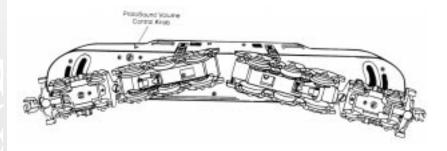
Figure 4: Adjusting The ProtoSound Volume
