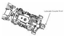
Figure 3: Lubricating The ProtoCoupler Knuckle
