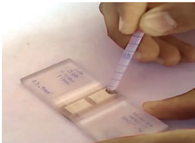
Fig. 13: Charging a chamber.
