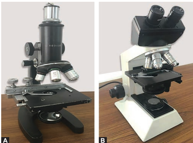
Figs. 1A and B: (A) Monocular microscope; (B) Binocular microscope.
