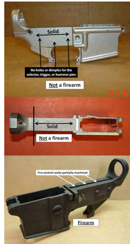
Images from the ATF website of some 80 percent lowers that can be transformed into fully-functioning firearms without serial numbers, https://www.atf.gov/firearms/ga/are-%E2%80%9C80%E2%80%9D-or-%E2%80%9Cunfinished%E2%80%9D-receivers-illegal .
