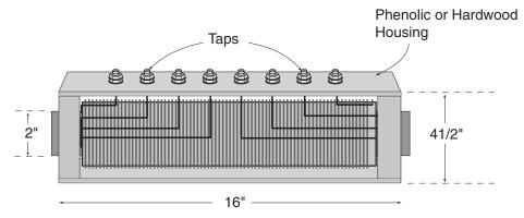
B. Ballast: Approx. 300 turns of #10 wire on a 2" dia. PVC pipe. Tap every 50 turns. If the system is to be operated on 120 Volts, use #8 wire.
