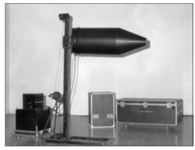
Fig. 1.1 - Tesla Coil and road cases. Oscillator lid (center) connects to wheeled base on Oscillator. Secondary Coil case (right) is fitted with hinged lid.
