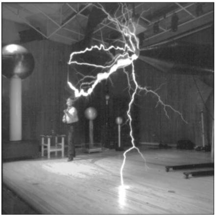
Fig. 38 - Performer draws a discharge to a grounded, hand-held aluminum rod. A constant, heavy discharge can be drawn up to about six feet. At greater distances, the discharge will wander.
