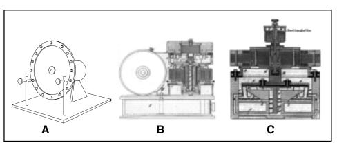
Fig. 4 - Rotary Spark Gaps. (A) Typical early design employing multiple points (B) Portable Tesla Mercury Interrupter attached to a Tesla Coil (C) Cross section of "industrial size" Tesla Interrupter.
