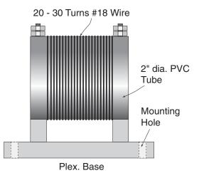
Fig. 44 - Radio Frequency Choke reduces RF
