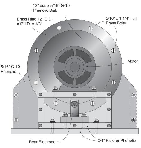
Fig. 24 - Rear View of Rotary Spark Gap
