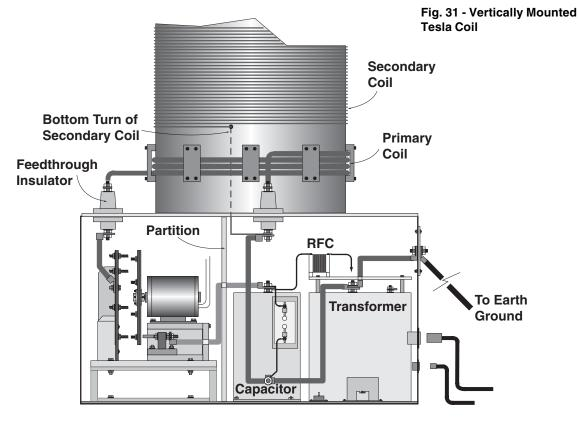
Fig. 32 - Parts Layout for Vertically Mounted Tesla Coil
