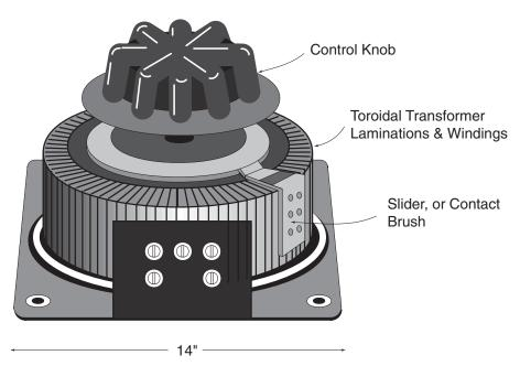
A. Typical variable transformer. Some units allow control knob to attach to either side, permitting flush mounting on a vertical or horizontal surface.
