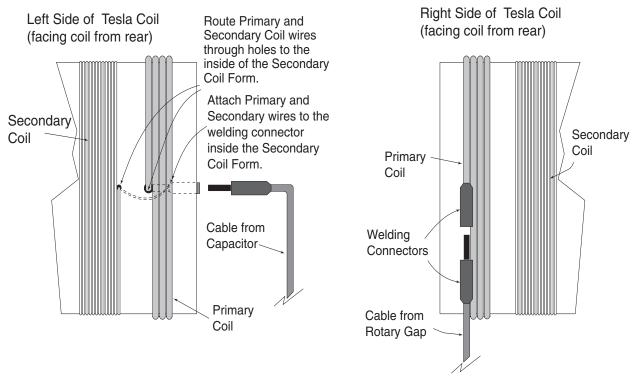
Fig. 13 - Primary & Secondary Connections
