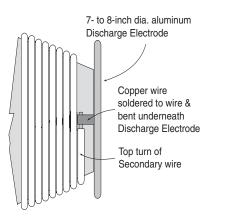
Fig. 12 - Secondary Winding Termination
