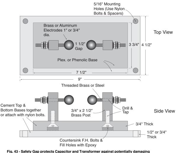
transient voltages generated in the Oscillator circuit.
