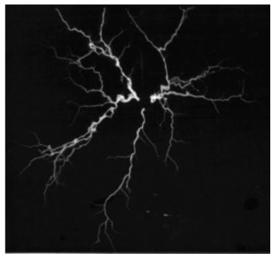
Fig. 36 - Discharge streamers eight feet long crackle from the Road Show Tesla Coil. Film exposure was around 1/3 second. A longer exposure would show more sparks, but this photo closely shows what the eye sees.
