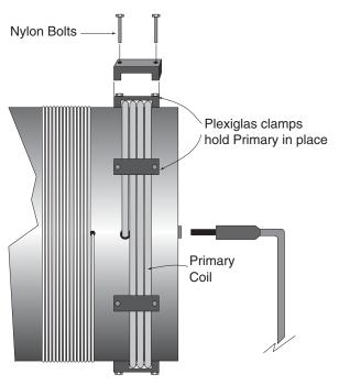
Fig. 14 - Securing Primary Coil
