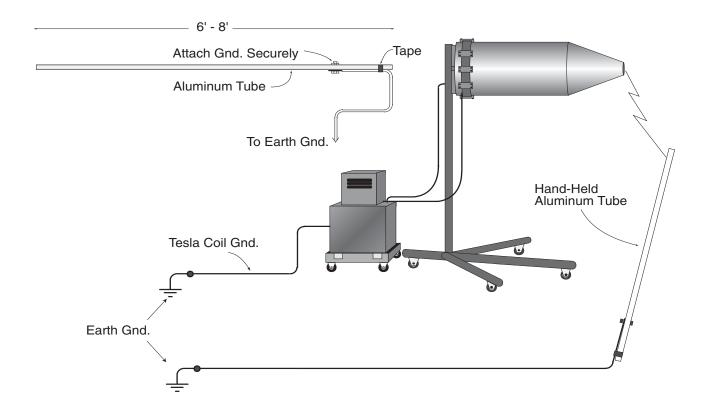
Fig. 37 - Hand-held Discharge Arrangement
