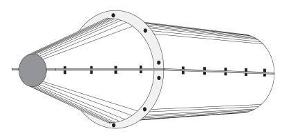
C. Assembled Mold Form With Connecting Flanges in Horizontal Position
