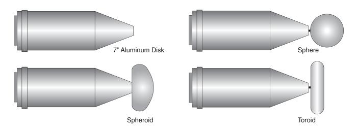
Figure 29 - Discharge Electrode Styles
