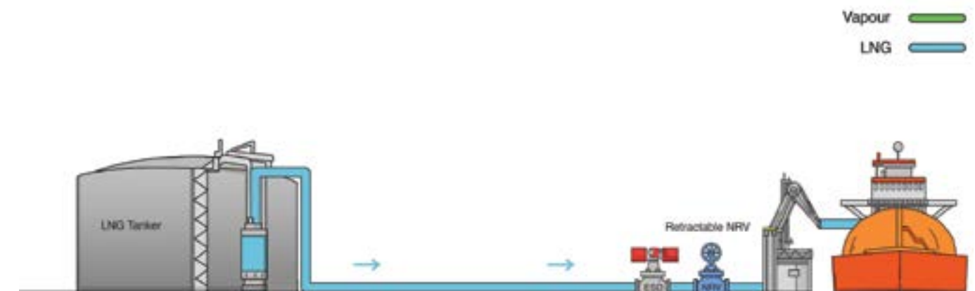
Figure 2.3 Illustration of a typical reloading operation with export into local infrastructure
