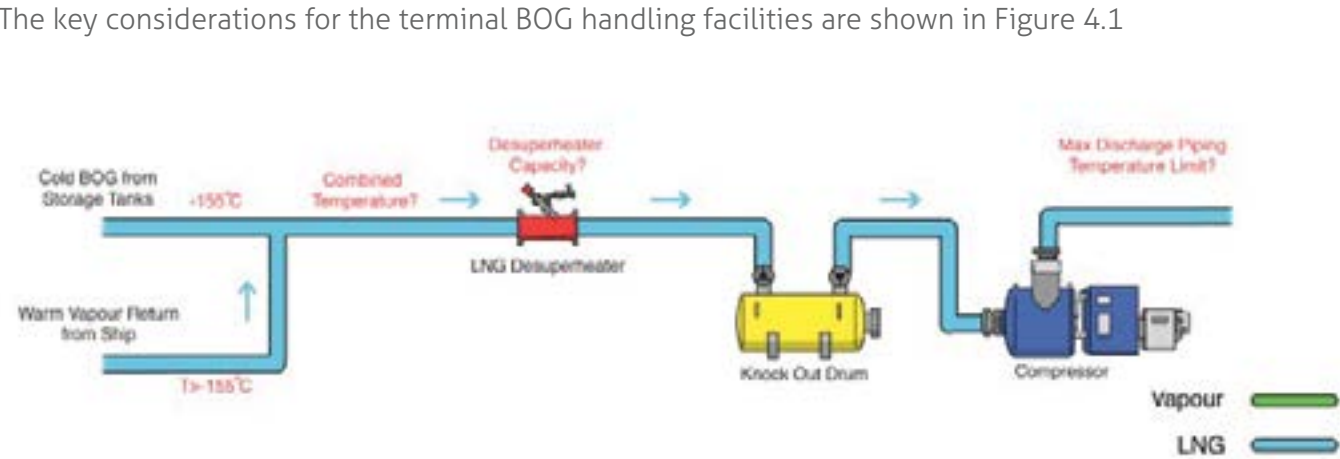
Figure 4.1 Illustration of typical factors to consider for terminal gas handling facilities
