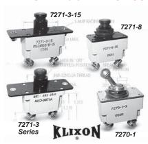
The Klixon 7270/7271 series circuit breakers were designed to uti-lize less behind panel space while protecting wire and cable in aircraft and ground support equipment on either 120 VAC. 400 Hz or 30 VDC systems. The units are available with neck mounting (7270-1 and 7271-8) or standard cover plate (7270-7 and 7271-(7270-7 and 7271-3). In each of these Klixon circuit breakers, the bi-metallic element assures uniform current distribution throughout
