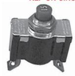
Feature a bi-metallic snap-acting disc as the sensing element. Widely used in production and military aircraft. The most popular models are illustrated. Models PSM and PSM-N are available in the following ampere ratings: 2, 3, 5, 10, 15, 20, 25, 35. When ordering specify if neck-mounting style is wanted by placing "N" after ampere rating.
