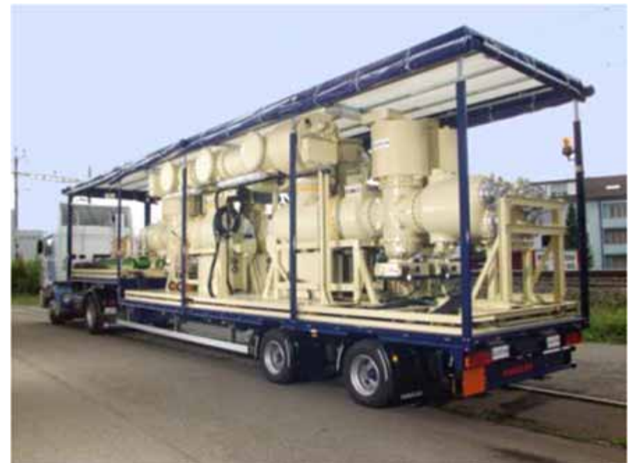
Spain – 145 mobile substation – 4 CB
